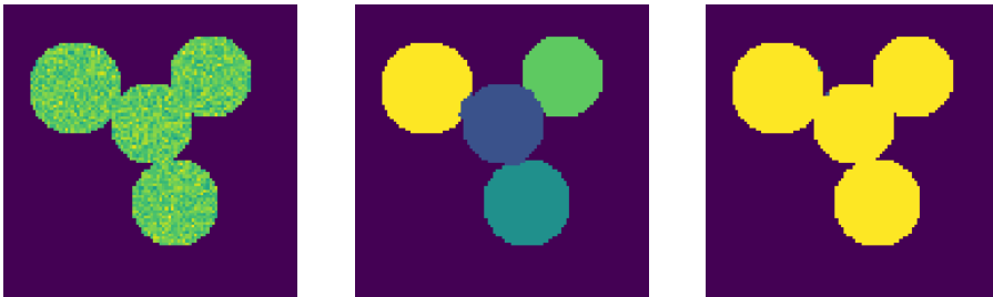
Figure: Normalized versus standard mincut segmentation: (a) a toy image with four circles (background masked out). (b) using spectral clustering on the four circles correctly identifies circles. (c) using mincut clustering on the four circles finds 3 segments of size 1. Trivial mincuts suggest a need to penalization for small segments.
